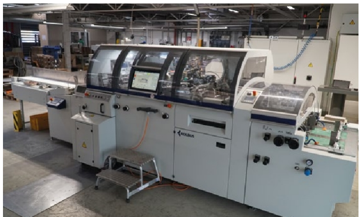
The all-purpose DA 370 ceiling machine represents the highest level of Kolbus engineering expertise. The Gutenberg Beuys fine printing company uses it to produce very high-quality books, such as art books.
