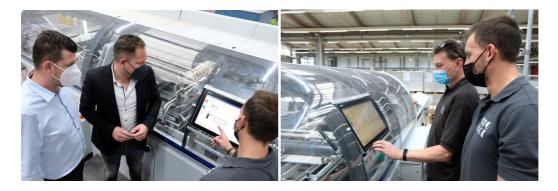
To meet production demands at Ludo Fact, Kolbus developed a new machine configuration linking two DA 290 inline casemakers complete with automated pallet feed and output stacking.
